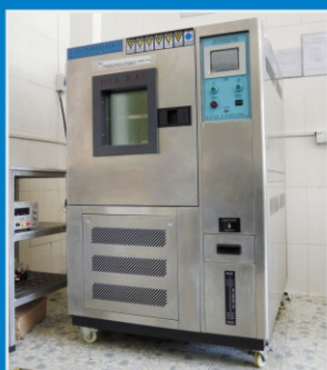
可程式恒温恒湿试验箱 Programmable Constant Temperature and Humidity Testing Chamber
